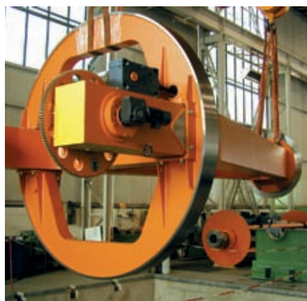
Workshop assembly of Drum Twister at Sket. Photos: Sket Verseilmaschinenbau
